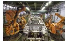
A photograph showing several industrial KUKA robotic arms working on an automotive assembly line. The robots are positioned around a vehicle chassis, performing tasks like welding or bolting. The background shows a factory environment with overhead lighting and structural elements. |
